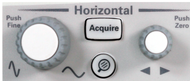
Figure 4 Oscilloscope horizontal (X-axis) controls
