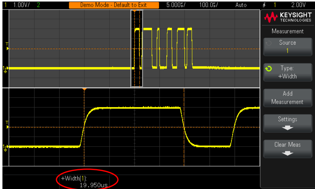
Figure 38 Using the scope’s Zoom timebase mode to perform “gated” measurements
