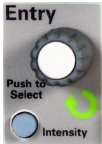
Figure 7 Oscilloscope general-entry control
