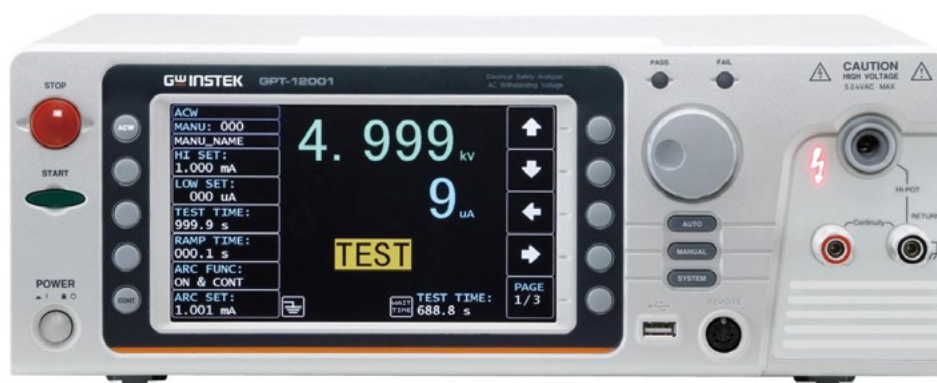
Fig 5: Electrical Safety Analyser
